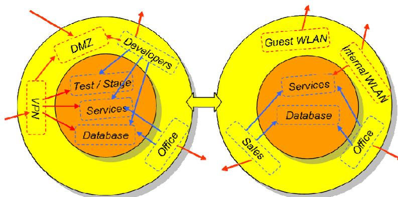
**Fig. 6:** Secure zones for small and medium environments
